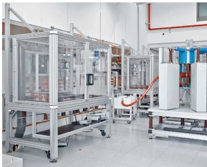
Fig. 25: Testing stations of the high-current testing system
